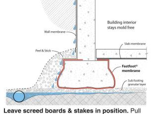
Fastfoot® off screeds and tape two edges together on top of footing with 2" sheathing tape.
