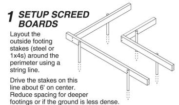
Drive inside stakes opposite each outside stake using a 1x2 cut to footing width. Top of footing is 3" less than the footing contact width (see diagram above right).
