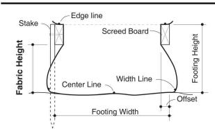
Using the edge line determined in step 2, staple corner edges to top of screed boards at 12" on center, using a hammer tacker with 3/8" staples.
